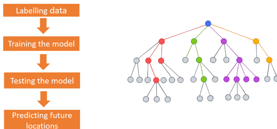
Figure 2: Four-step process of the Random Forest algorithm.
